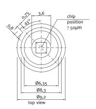
UVC-only SiC based UV photodiode A = 7.6 mm<sup>2</sup>
